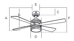
A. Top of Canopy to Bottom of Blade 44 cm B. Top of Canopy to Bottom of Switch House 50 cm C. Top of Canopy to Bottom of Canopy 6 cm D. Width of Motor Housing 19 cm E. Width of Canopy 13 cm F. Top of Canopy to Bottom of Glass / cm
